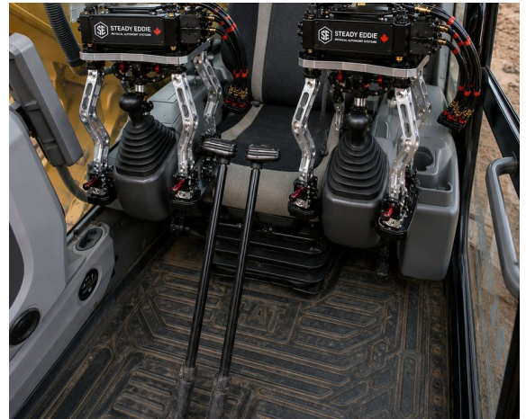
AN EXCAVATOR'S OPERATOR STATION, THE WIDE VIEW. THE DOCK IS FITTED ONCE, MECHANICALLY
